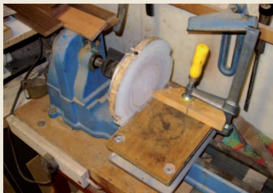
Prototype Andrew's first disc sander was nothing more than a chipboard disc mounted on a lathe chuck, with a table bolted to the lathe bed
